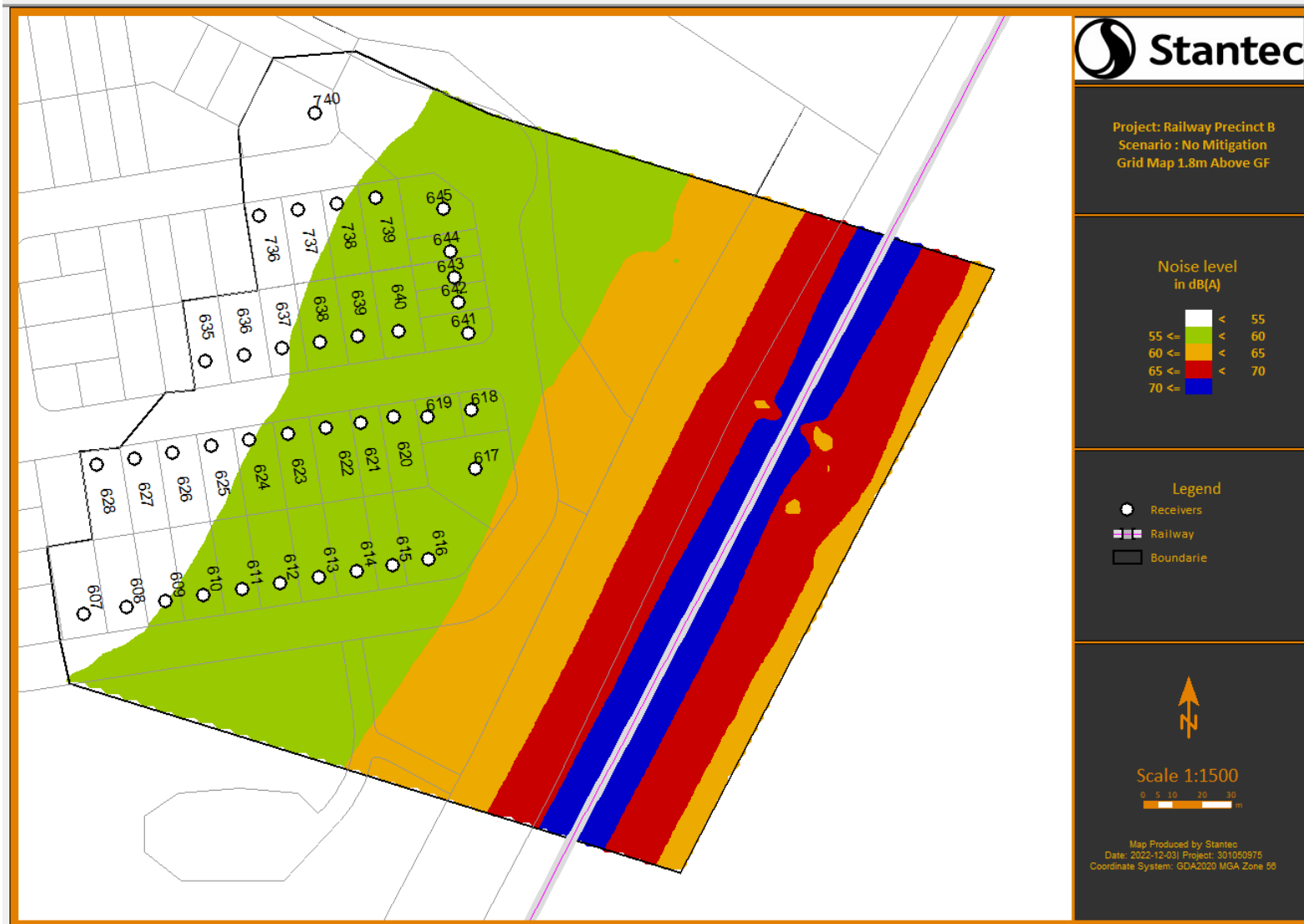
Figure 8: Predicted Rail Noise Levels – Ground Floor Level
