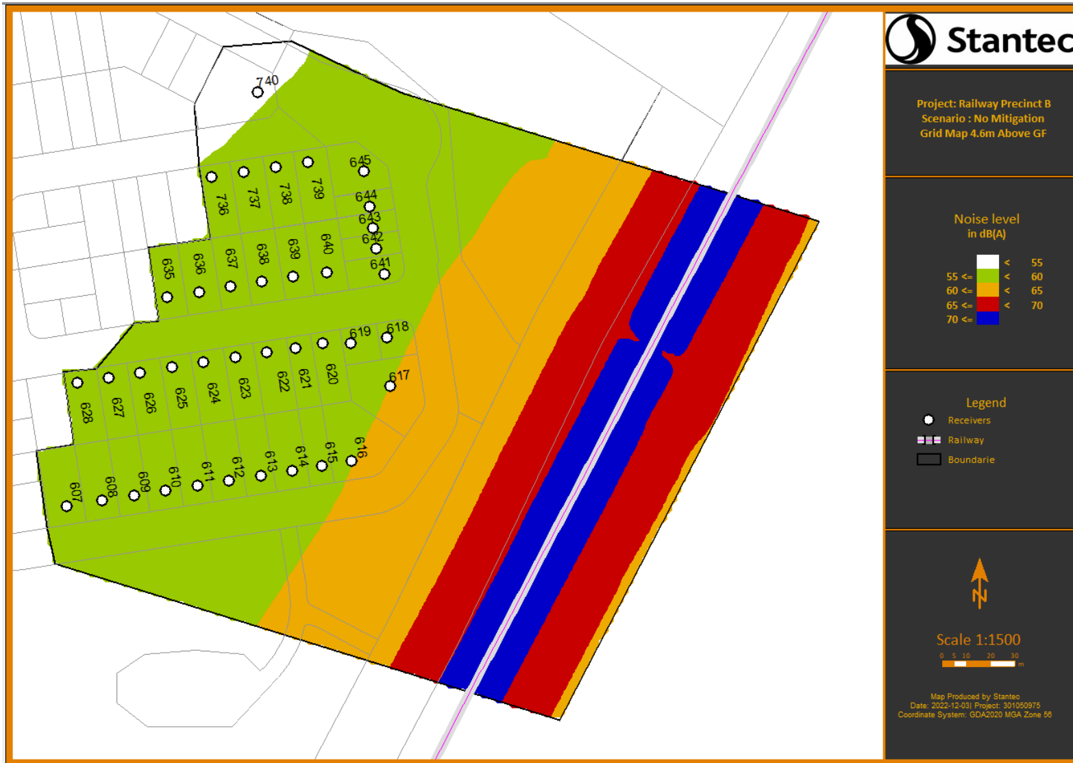
Figure 9: Predicted Rail Noise Levels – First Floor Level
